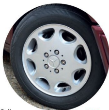
ABOVE 'Eight-hole' alloys were fitted for the last four years of 124s.
