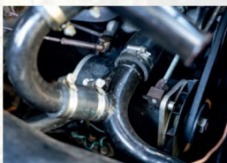
ABOVE Tim replaced the dynamo, which boosts electrical charging.
