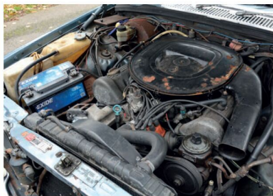
BELOW 77 M117 has mechanical injection, better than the earlier electronic setup.
